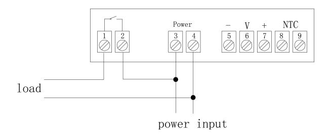
erminals 1 and 2: Normally opened contact of relay Terminals 3 and 4: Connect the power Terminals 5 and 6 and 7 : Connect the Humidity sensor Terminals 8and9: Connect Temperature sensor
